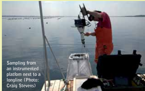
Turbulence profiler about to be deployed next to a longline (Photo: Craig Stevens)
